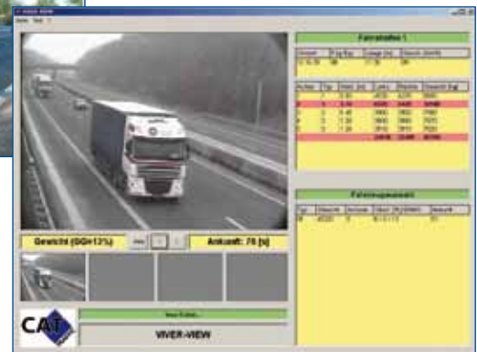
Weight Enforcement Network Germany with UMTS-based Video Preselection
