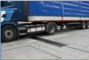
Bending Plate Site
